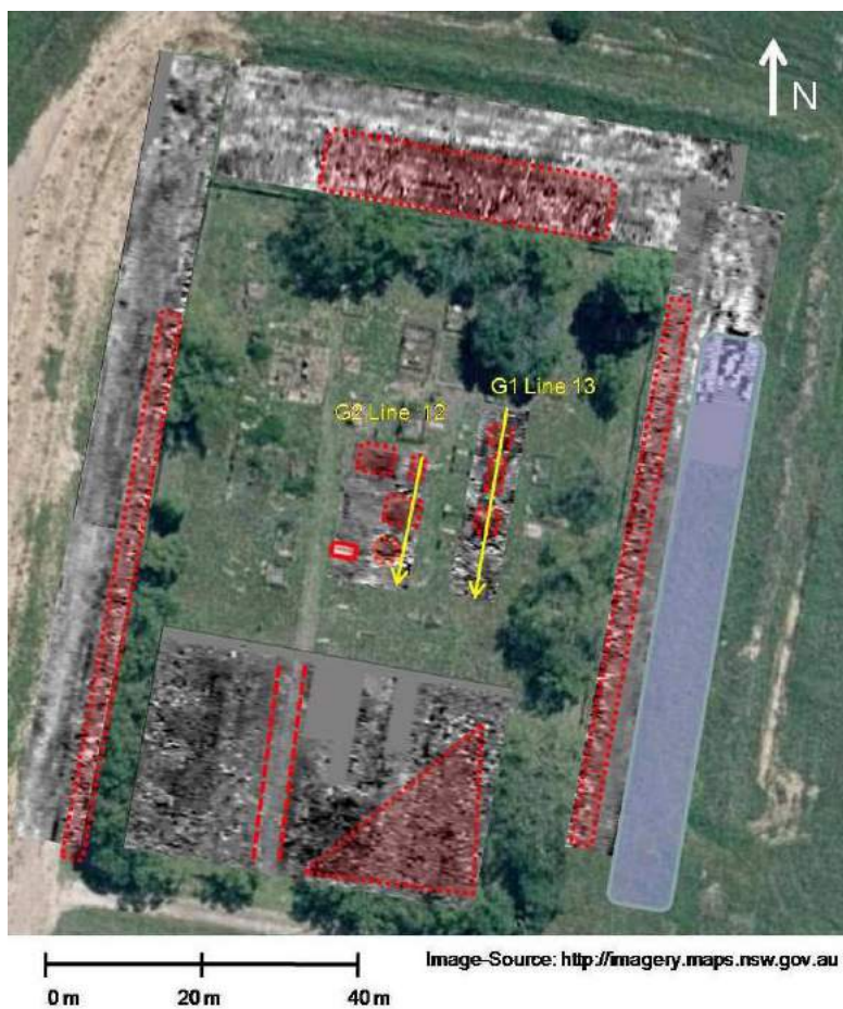
Figure 13 GPR survey results. The path's historic location was confirmed. The southern third of the site may contain graves, especially the triangle. (Source: ACL)
